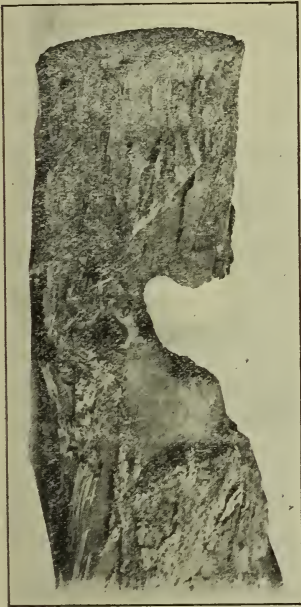
Fig. 23. Showing burning caused by alternating current wire.
